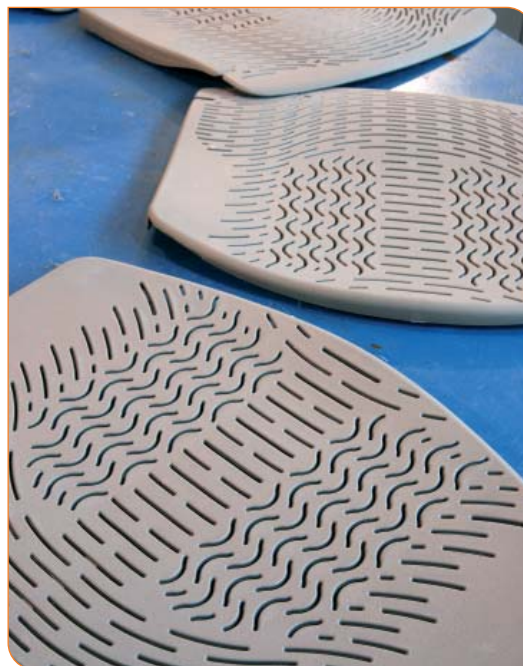
Life Chair seats coming out of the injection moulder. Axiam Plastics has been making the moulded plastic seats for Formway Furniture since 2005.
