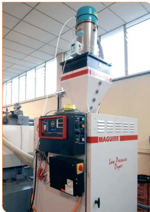
The resin particle vacuum drier in operation. The dried plastic granules are transferred by vacuum loader to the injection moulder behind.
