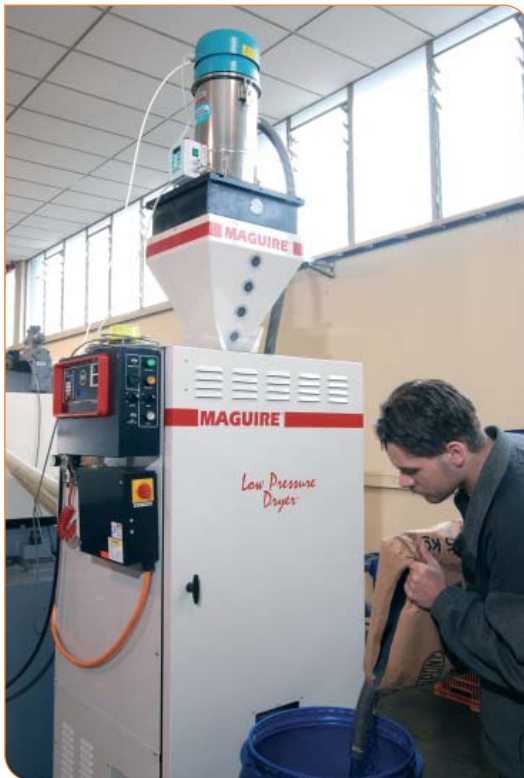
Darrell Sanderson loads plastic granules into a feeding bin, ready to be sucked into the resin particle vacuum drier.
